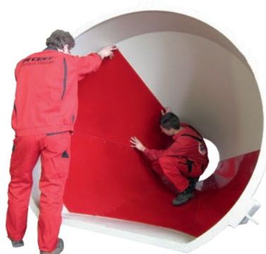
The liner was fitted into the hopper
