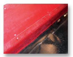
It is a combination of PUCEST sheets with and without a perforated plate. Perforated plates are used for attachment and stabilization. The pure PU-part has through its tension a light contact with the conveyor belt and it is self-adjusting, so that no material falls down to the left and to the right. The wear protection can be combined together with other PUCEST panels with any height and length
