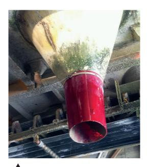
A PUCEST discharge hose after a wear life span of 100,000 m<sup>3</sup>
