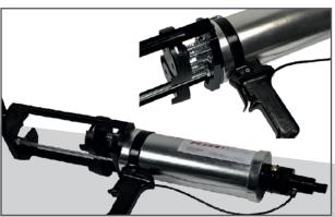
For an optimal performance we recommend an air pressure from 102 to 116 psi / 7 to 8 bar.
