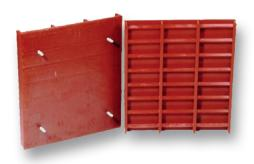
This PUCEST pocket panel works on a simple principle: A portion of the conveyed material, which on the plate rebounds, accumulates in the chambers and thus assumes a buffer function. The wear effect is slowed significantly this way. A further advantage of the baffle plate is its elasticity. Coarse grained goods (for example gravel) does not crack when collision. The use of PUCEST pocket panels with material buffer is recommended when using a grain size up to 32 mm.
