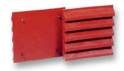
The standard size of the plates is 500 mm x 500 mm with a thickness of 50 mm. The shore hardness should be chosen by customer between A 50-95°. Baffle plates can be quickly and easily installed using stay bolts on the back side.
