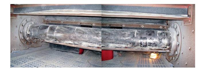
Protective pipe of the eccentric and the traverse inside of separating plant is subject to substantial wear and its working durability often predictable. The replacement or repair of these protective pipes is oftenvery complex and that's why it can raise significant costs and production downtimes.
