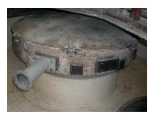
Adapter plates are welded. The console is fixed by four bolts as the spring unit. The arm and the mix blades are installed.
