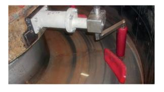
In order to reach a faster emptying a clearing strip can be installed. For small parts it takes more than 15 minutes to be changed. Easy installation of the mixing arms and blades allows the system operator to perform this at the same time. Optimally installed mixing instruments mean less cleaning works and reduced wearing of blade and body.
