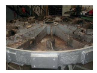
Mixing arms, spring elements, control levers and other parts are removed from the removed. Arm open end holes are closed by a plate.
